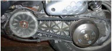
Now we have to take off the clutch bell (or clutch housing). You can use an impact wrench or standard hand tools to unscrew the nut. With hand tools, you will need an oil filter chain or strap wrench to hold the bell. Turn in the direction shown in the illustration.
