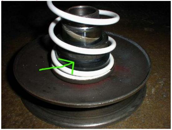
To change the clutch springs, use a screwdriver. Depending on scooter model their is usually 2 or 3 springs.
