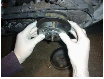
Put on the bell and tighten it to the proper torque. Follow the arrows in the picture .
