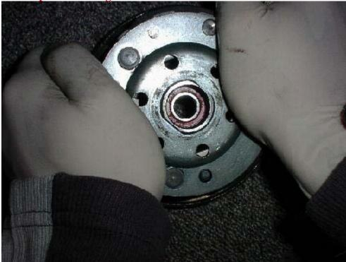
Reinstall the nut to the proper torque. Standing on the assembly will help.
