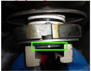
Then use you oil filter chain to turn the clutch so that the nut will come loose.
