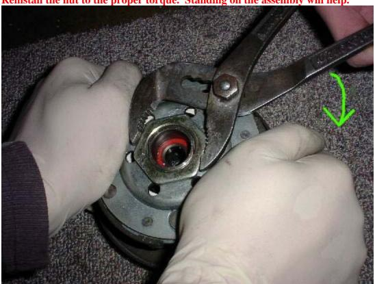
Reinstall the clutch. Squeeze it again to get the belt on before installing.
