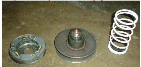
To change the torque spring you only have to replace it and rinstall the safety bolt (if there was one).
