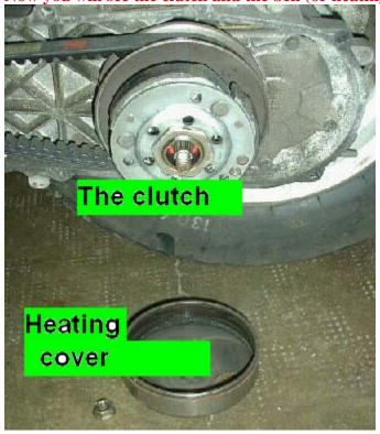
Squeeze the clutch pulley halves apart. The belt will become slack and loosen, then you will be able to take out the clutch assembly.
