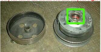
To take out the clutch nut you will need to put it in a vise. Don't tighten it too tight - just enough so that it is held firm.
