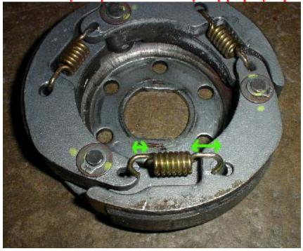
To put them back together, use a screwdriver or a pair of pliers. Watch your fingers - the springs are under tension.
