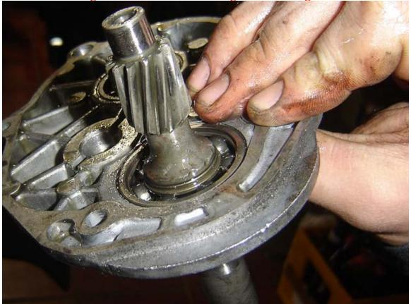
You need to take out the bolt that's in the big shaft. I used a rubber hammer.
