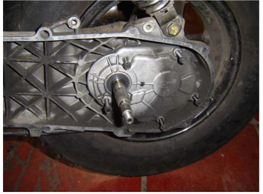
Don't forget to put a pan underneath so that the transmission oil doesn't go on the floor and make a mess like I just did
