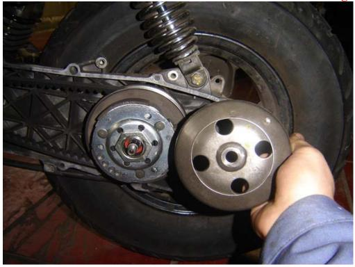
The clutch shoes are on the left and the clutch bell is on the right
