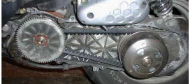
Unscrew the clutch nut with an impact gun, or an oil filter chain or a strap wrench (you can find these all hardware or auto stores). A strap wrench is shown in the picture. You won't need this with an impact wrench.
