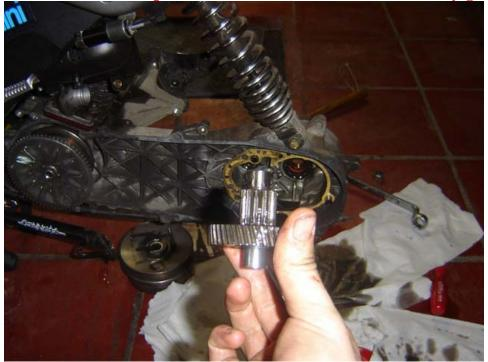
You can remove the gear using a rubber mallet. The lower gear is net being held tightly in the vise - it is free to move.
