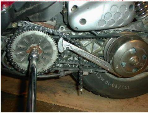
This is what you would get after taking off the variator cover. The variator is in back of the belt. To get the variator out, just slide it off the shaft.
