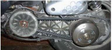
Unscrew the variator screw with an impact gun or an oil filter chain (You can find at all hardware stores). Use the technique in the picture to open it faster and
